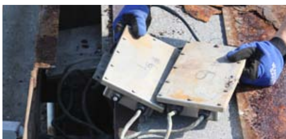
Junction boxes contain circuit boards and many manual wire connections. They are the main cause of truck scale downtime because they are difficult to seal against moisture
