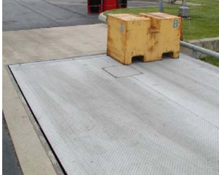
A test weight on scale corner
