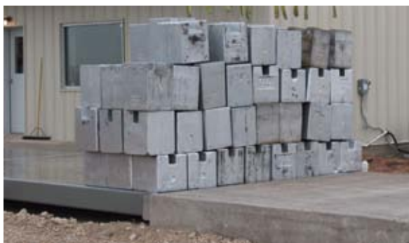
Test weights on a truck scale
