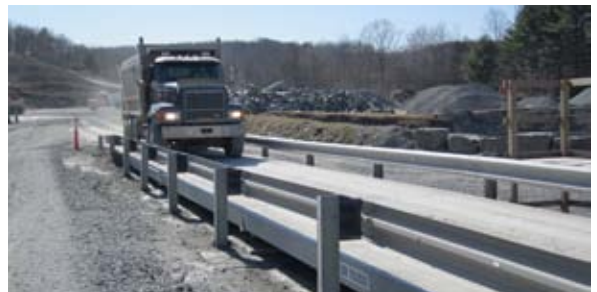
These stand-alone guiderails are planted in the ground alongside the scale to offer added strength and prevent trucks from driving off the side of the scale
